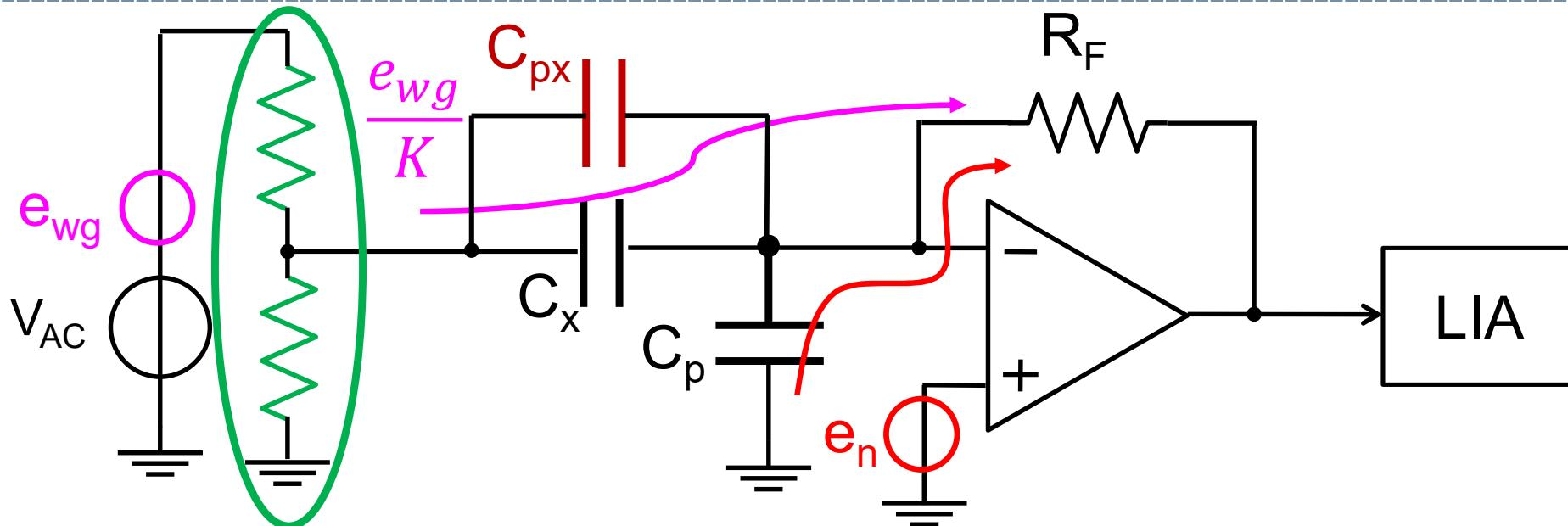
Voltage divider using small value resistors ( $\approx 50\Omega$ )
